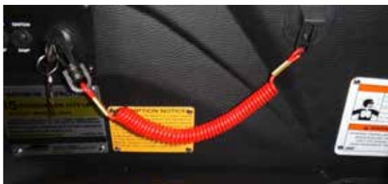
clip will pull free, pulling the switch to the OFF position. If the engine needs to be shut down very quickly, it can be done so by pulling on the lanyard to release it from the switch.
