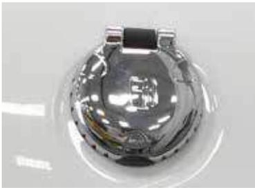
Axis boats are equipped with fuel fill fittings and vents to provide state-of-the-art safety protection in the process of adding fuel to the tank. While most of the fuel system on the boat is inaccessible to owners/operators, the fuel fill was designed to ensure the process of fueling up is as safe as possible and efficient.
