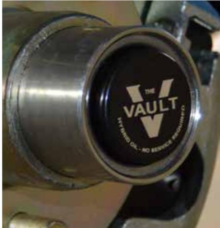
A slight amount of oil seepage at the rear seal is normal and necessary to lubricate the wiper lip of the seal for long life and sealing contaminants out. If excessive leakage is occurring, however, contact an authorized Axis trailer dealer.
