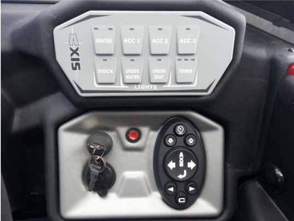
**Heater:** Press this button once to turn the Heater ON with the blowers operating on HIGH. The LED on the left side of the button will light. Press the button a second time to reduce the blowers to LOW. The LED on the right side of the button will light. Press a third time to turn the Heater OFF.
