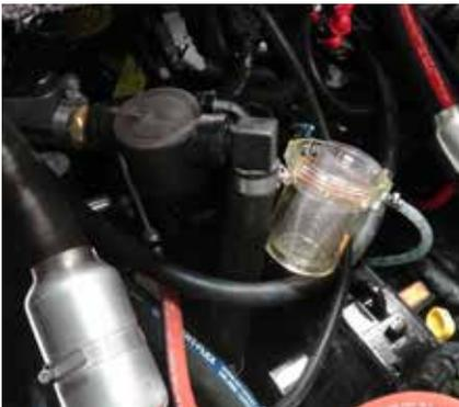
When operating the boat in "dirty" water that is brackish or has a noticeable degree of weeds and other flora, it may be necessary to clean out the strainer in boats equipped with sea strainers even during an outing. Pay close attention to the engine temperature, which appears on a gauge. (See the *Instrument Panel and Gauges* section of this Owner's Manual for more information.) An overheating engine is probably due to inadequate water flow.
