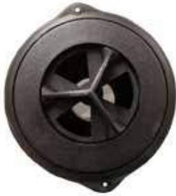
A popular option on all models is the heater. Warm air is blown through a liquid/air heat exchanger using hot water or coolant from the engine. Vent locations vary by model, so owners/operators and passengers should familiarize themselves with the locations. The vents have sliding, directional gates that can redirect the air flow, or even shut it off.
