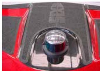
Bow lights are located at the front of the bow. On a traditional bow, it is two-colored—red and green and operated from a button on the dash panel.
