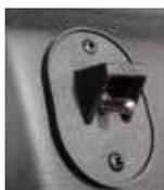
The Emergency Engine Stop Switch attaches to the boat operator by way of a lanyard for the purpose of shutting off the engine if the operator, for any reason, moves or is moved away from the driver's helm.
