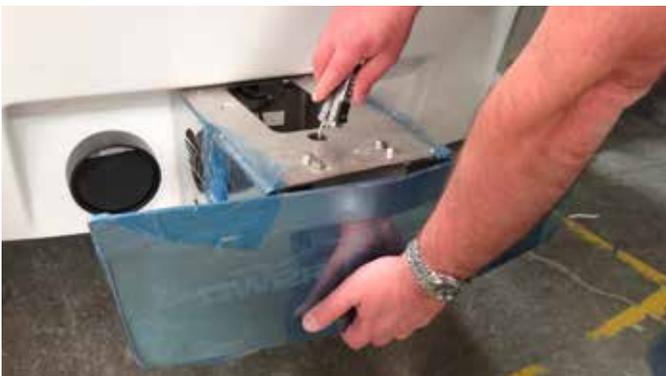
For the Power Wedge, using a small (stubby) straight screwdriver, loosen a small red screw on top until it stops. Lift or lower the wedge to the position desired and then tighten the screw snugly (but do no over-tighten). Manually cycle the wedge a couple of times after doing to ensure that the screw is snug and the wedge moves correctly.
