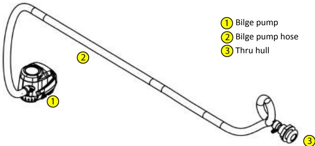
If water ever enters the forward part of the bilge, it can still be evacuated by the bilge pump. Located in the forward berth, there is an inspection plate, when removed, allows access to a drain plug. Simply remove the drain plug in the PVC pipe to allow the water to drain aft. Once all of the water has drained, re-install the drain plug.
