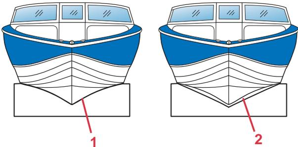
1 – Hull completely on cradle — right
