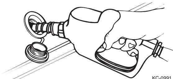
When your boat is equipped with the pop-up fuel filler cap, open by pressing the cap and turning the cap counterclockwise (approximately 10°); remove cap.
