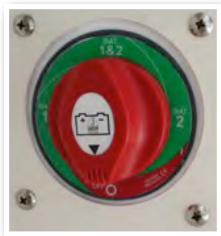
Battery Switch, Shown in the "Off" Position
