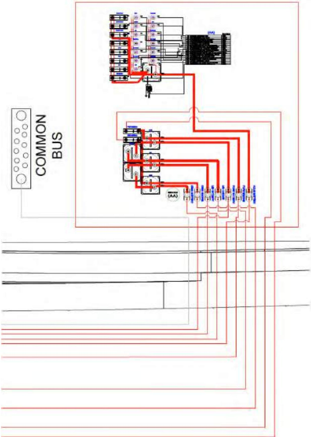
344 Power distribution diagram for leaning post/ batteries
