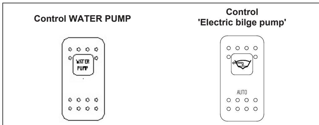
On the electrical panel - three possible positions : OFF / Automatic / Mechanically operated.
