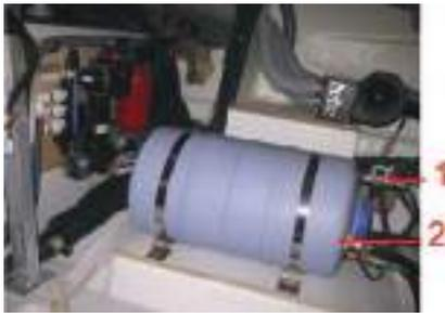
Operation: The water heater works off the starboard engine system + on 220V.
