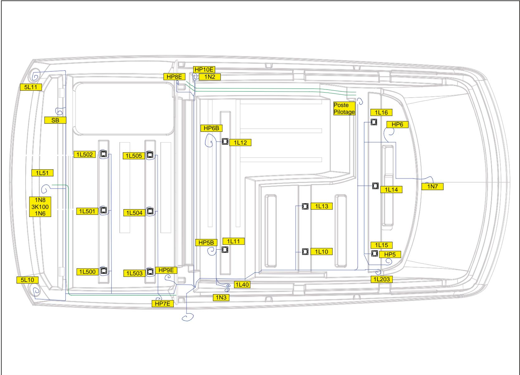
7.2.8 Diagram of flying bridge wiring looms - DC circuit
