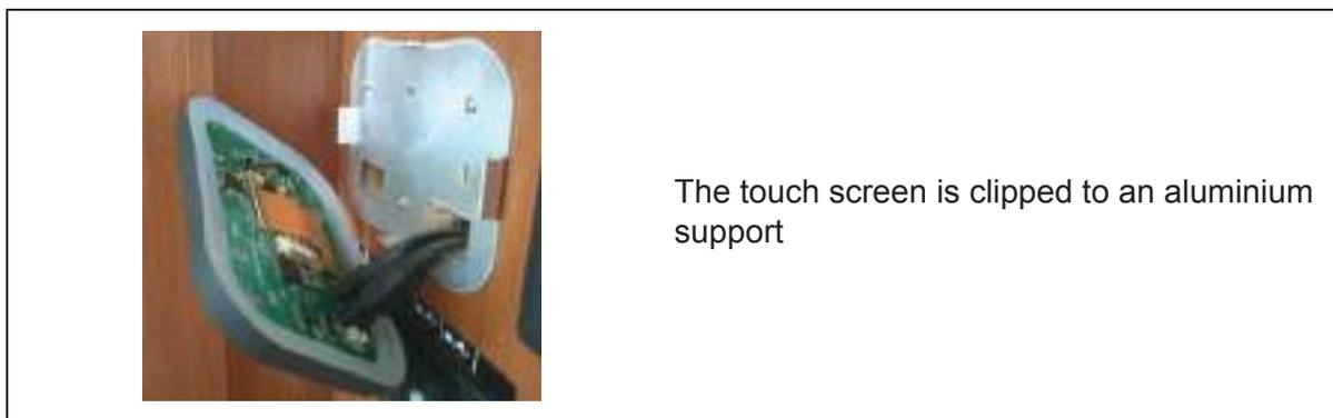
The touch screen is clipped to an aluminium support
