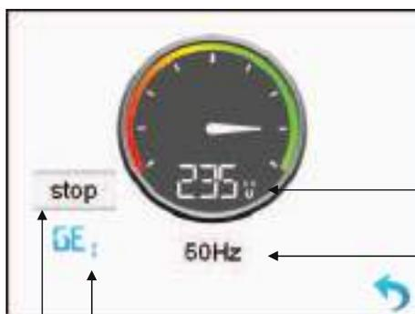
Voltage provided by the generator for on-board supply
