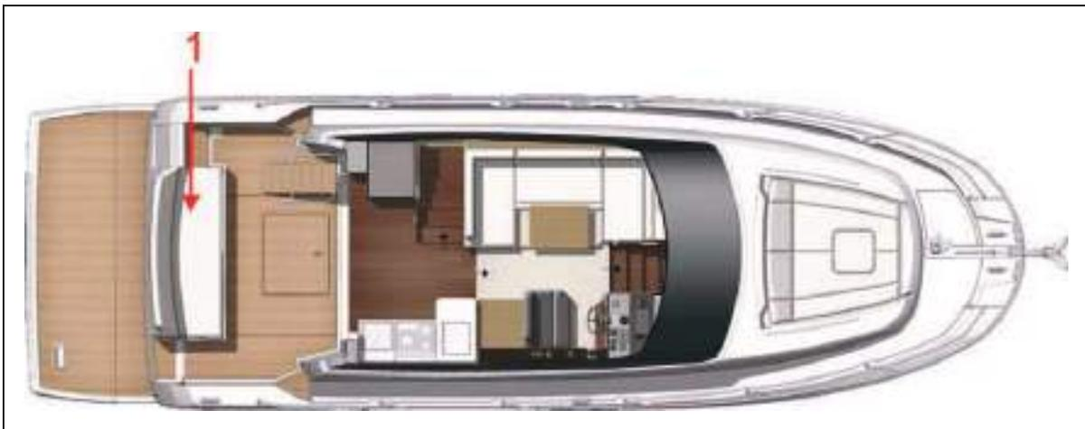
The life-raft(not supplied) must be stored in the space provided for it (Ref 1). A pictogram helps to locate it easily.
