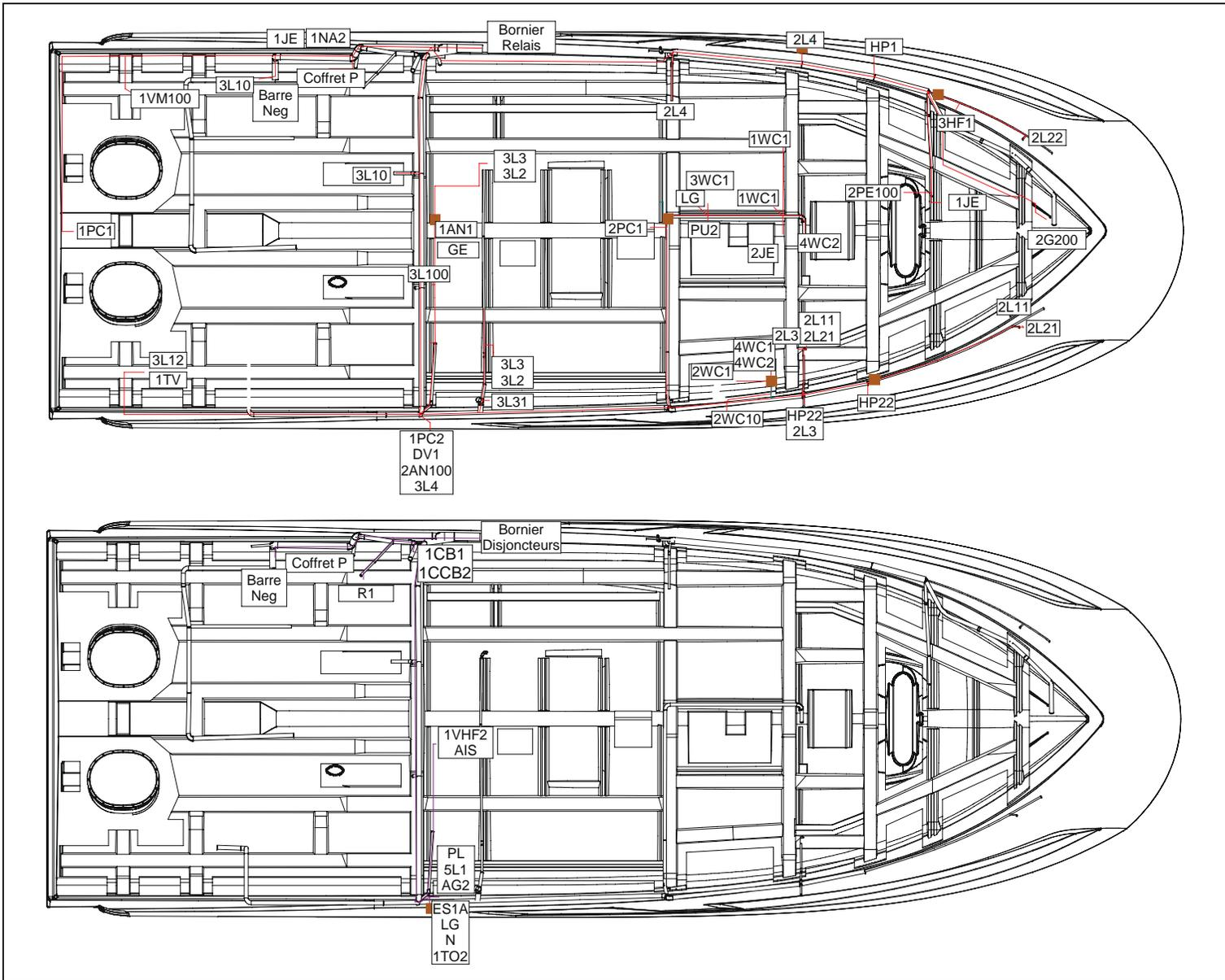
7.2.6 Layout of the wiring looms in the hull - DC circuit
