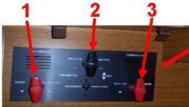
1. Battery switch + Engine
