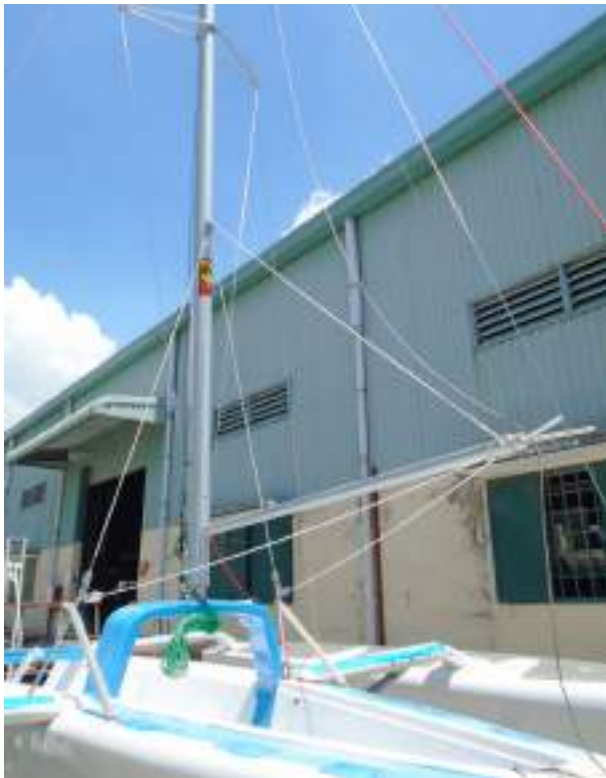
Mast on way up and being held from going sideways by raising wires
