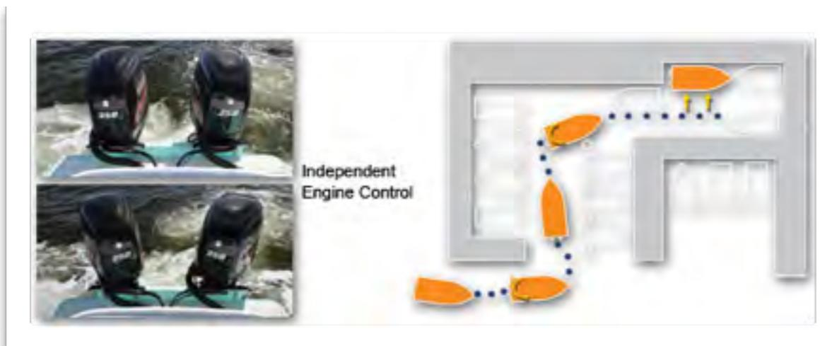
trailer. Even novice boaters using the Optimus 360 Joystick Control System can confidently move the boat forward, backwards, diagonally, rotate it on its own axis, or even move sideways to accomplish tricky docking maneuvers. As the operator easily moves the joystick, the SmartCylinders and actuators respond instantly to independently steer each
