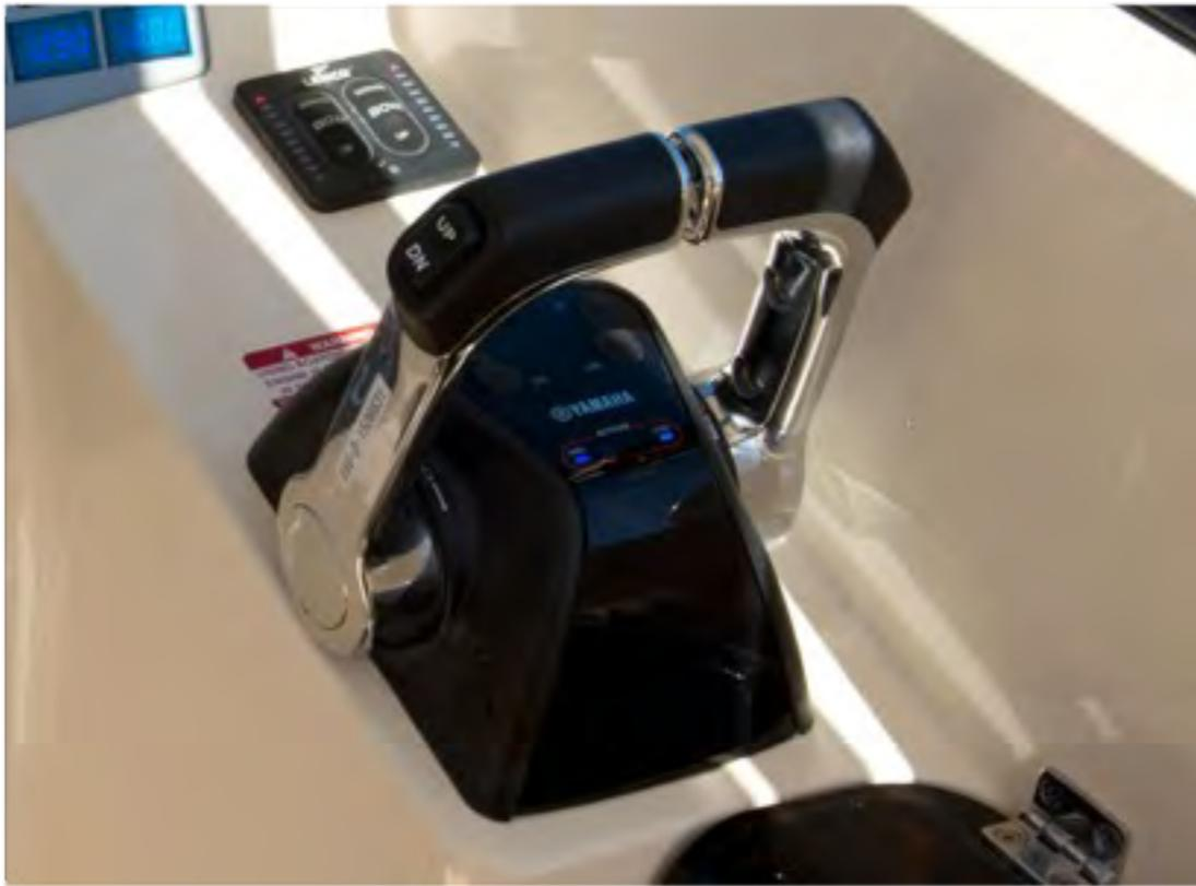
the shift lever is in any position other than the neutral position and should be inspected and tested periodically to ensure the switch is working. If an engine will not start, slight movement of
