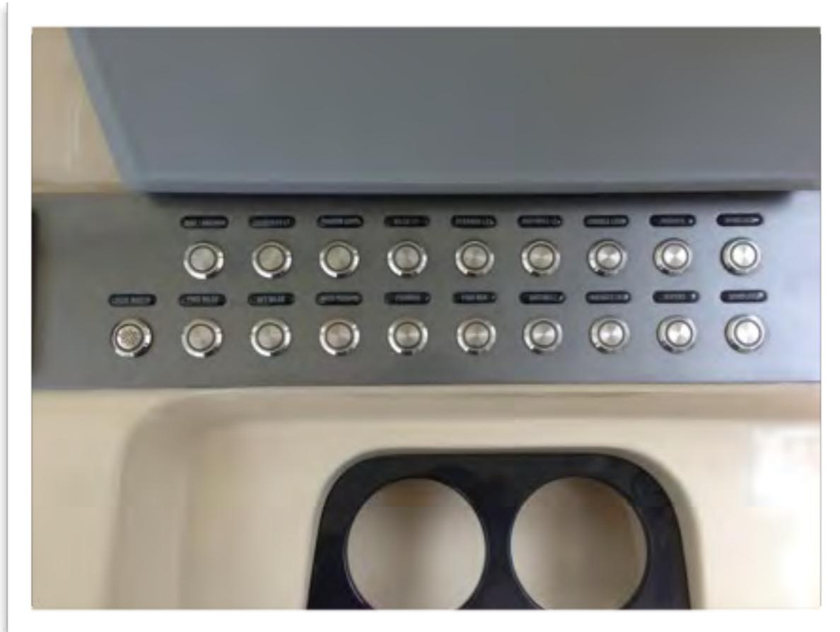
This switch controls the windlass which is mounted in the anchor locker. It is protected by a circuit breaker of the type and rating recommended by the windlass manufacturer that is located near the battery switches.
