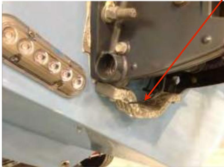
occurs is relative to the water conditions in your boating area. Water temperature, pollution, current, etc. can have an effect on marine growth.
