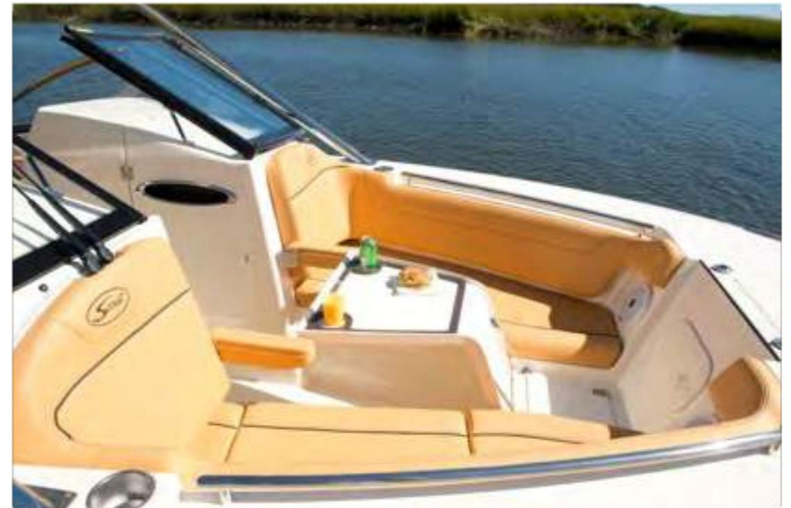
Seat cushions are secured to the hatches with snaps.
