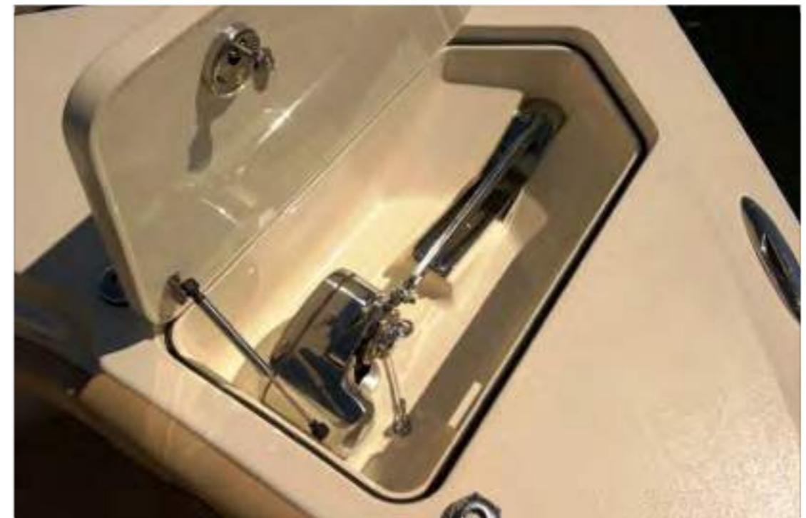
The anchor line is always stored in the locker. If the anchor is stored in the anchor locker, it must be properly secured to prevent it from bouncing in the locker and causing damage to the hull or anchor locker.
