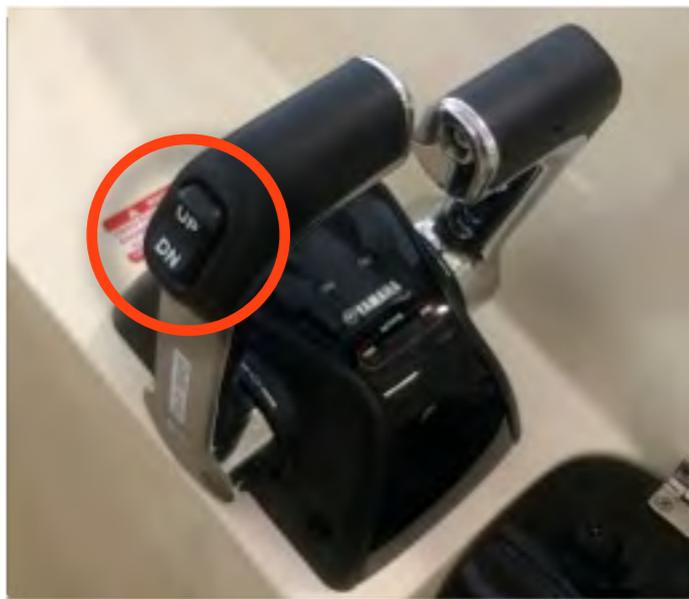
Some engine controls have two switches on the control cover to activate each engine individually.
