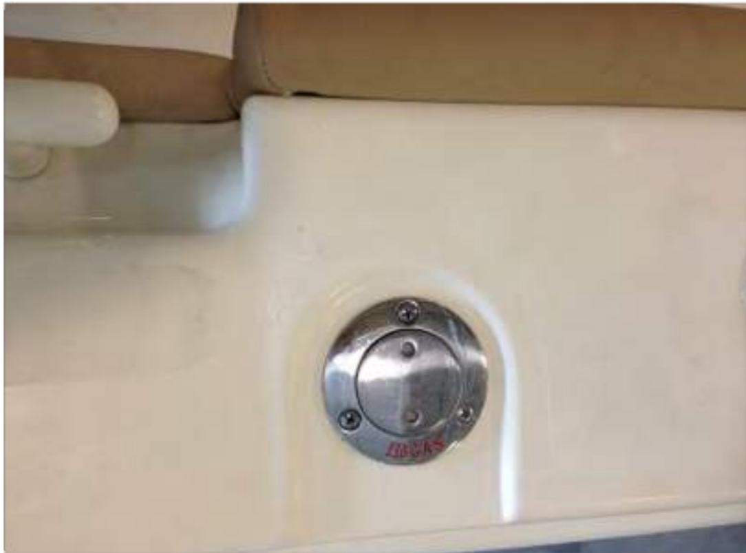
**Note:** Do not over-tighten the fuel cap. If the cap is overtightened, the O-ring seal could be damaged allowing water to contaminate the fuel system.
