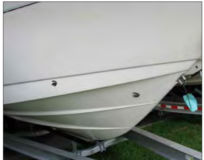
Bow Storage Compartment & Rope Locker Drains
