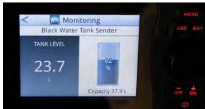
Tank Level Monitor
