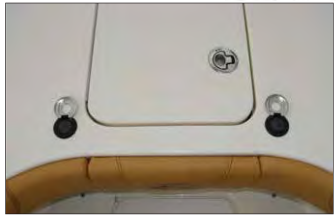
Windlass Foot Switches & Safety Covers
