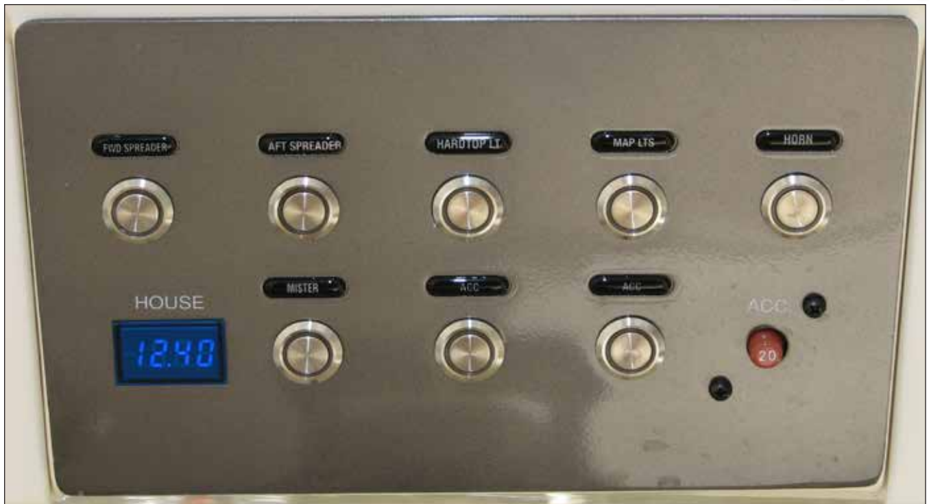
Hardtop Switch Panel, House Battery DC Volt Meter & Accessory Circuit Breaker
