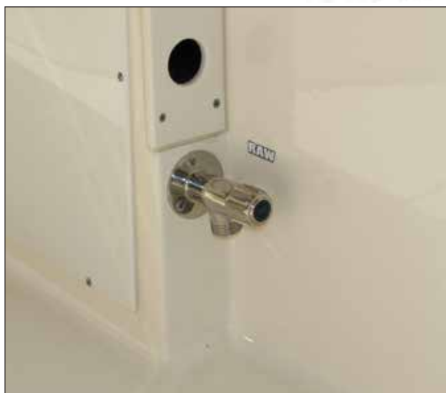
Cockpit Raw Water Washdown Connection
