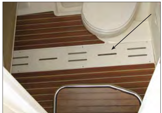
Removable Grate To Access Forward Bilge
