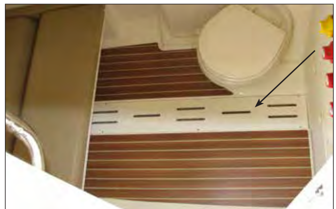
Cabin Sole Drain Grate
