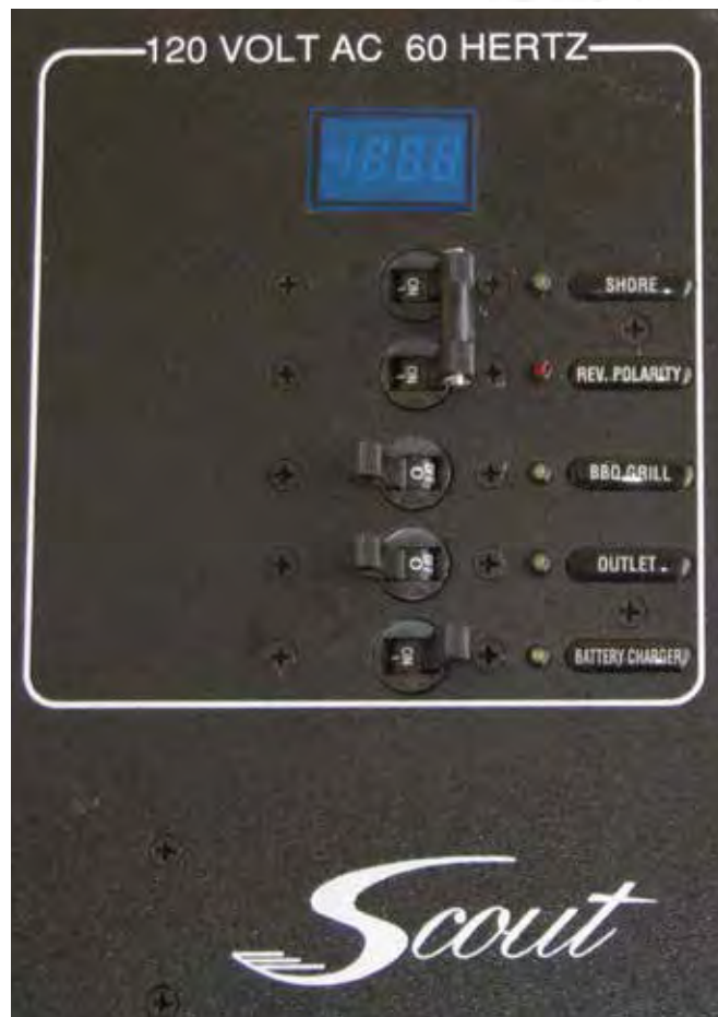
AC Circuit Breaker Panel
