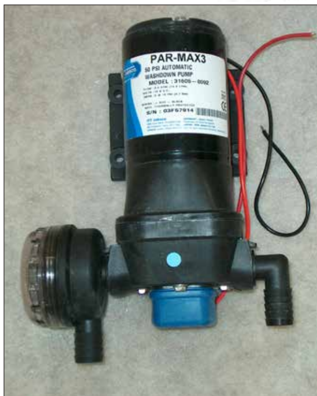
Raw Water Washdown Pump & Strainer
