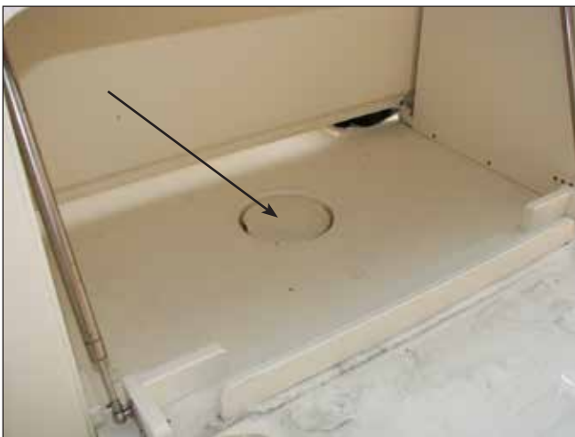
Fuel Tank Level Sending Unit Access Hatch
