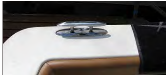
Stern Mooring Cleat Up
