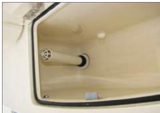
Leaning Post Baitwell Standpipe & Drain Fitting
