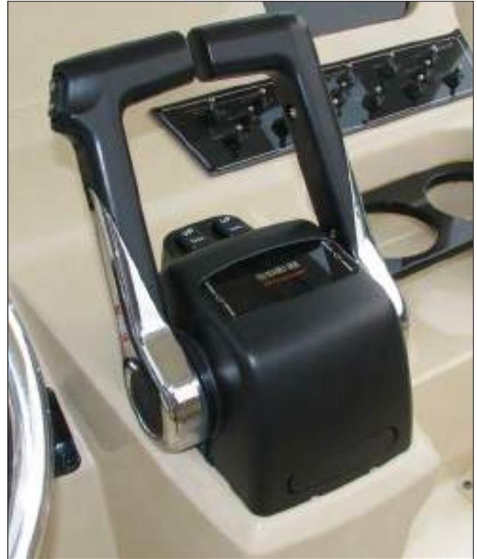
Typical Twin Engine Cable Controls
