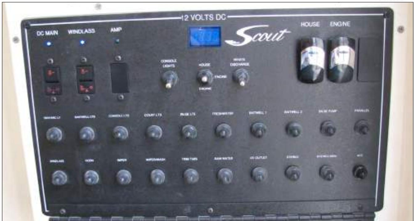
DC Breaker Panel & Remote Battery Switches
