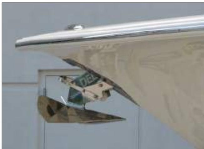
Anchor Roller & Delta Plow Anchor
