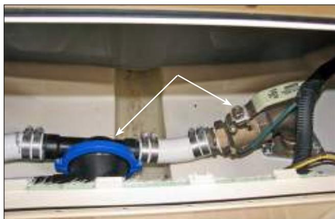
Waste Discharge Pump & Thru-Hull Valve
