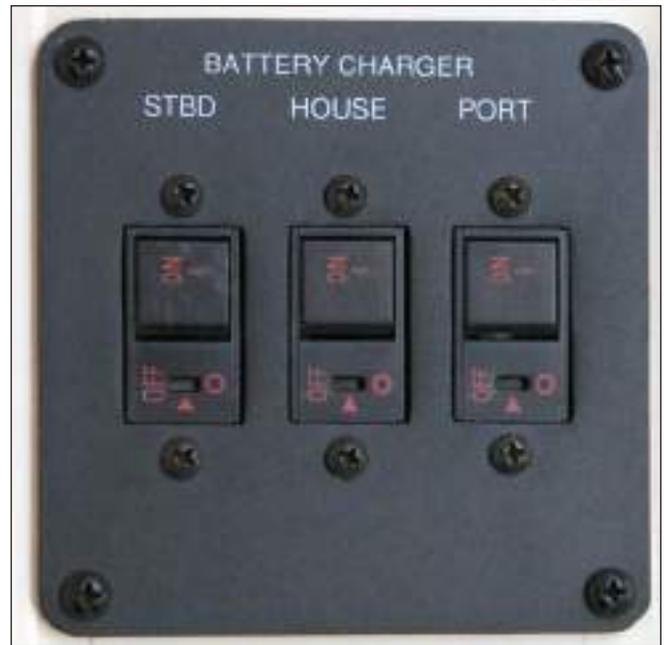
Twin Engine External Battery Charging Circuit Protection
