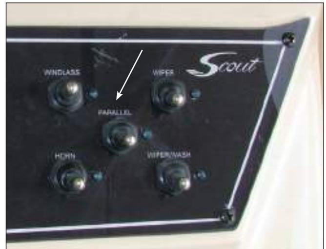
Parallel Switch In Helm Switch Panel
