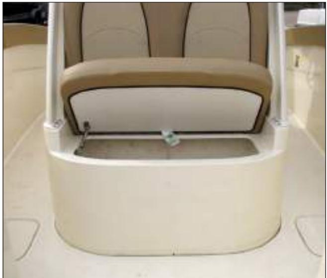
Forward Console Seat Cooler Hatch
