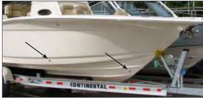
Forward Fishbox/Storage Compartment & Rope Locker Drains
