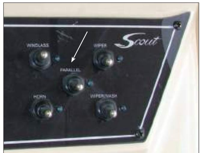
Parallel Switch In Helm Switch Panel
