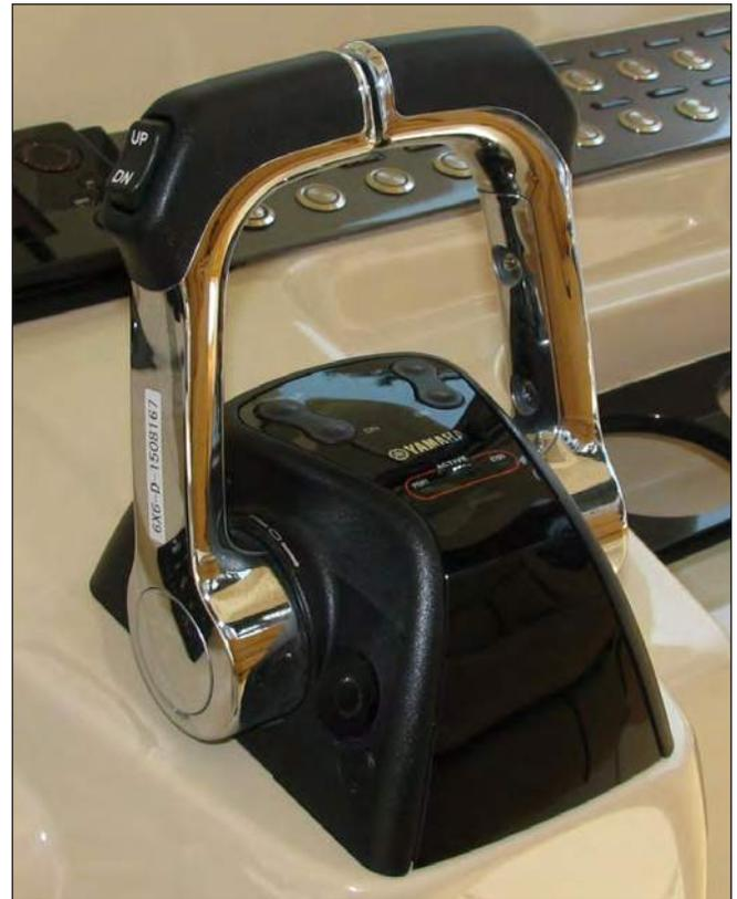
Typical Yamaha Twin Engine Electronic Controls
