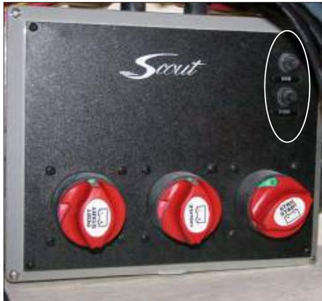
Twin Engine Battery Switch Circuit Breakers
