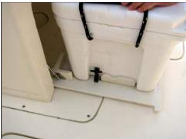
Cooler Slide Assembly & Draw Latch
