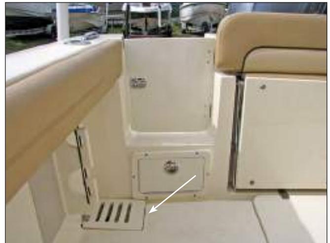
Starboard Cockpit Scupper Drain
