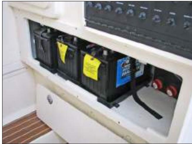
Typical Twin Engine Batteries
