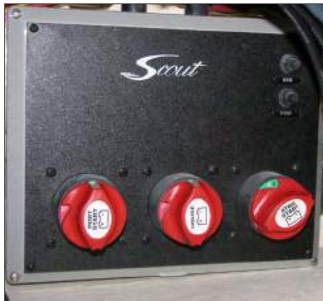
Twin Engine Battery Switch Panel
