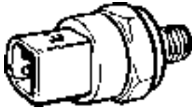
Fig. 122. Oil pressure relay
