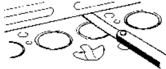
Fig. 15. Checking of cylinder head flatness
