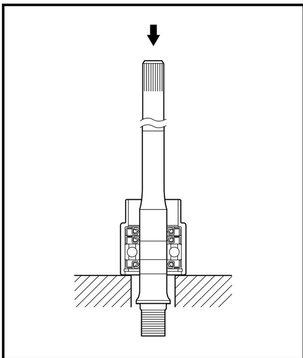
**Intermediate drive shaft removal**
