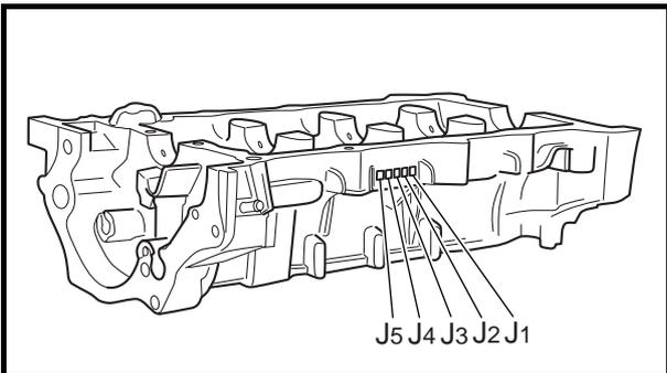
For example, if the crankcase “J1” and crankshaft web “J1” numbers are “8” and “2” respectively, then the bearing size for “J1” is:
