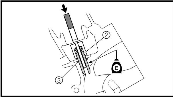
2. Install the new valve guide ② by striking the special service tool from the camshaft side until the valve guide clip ③ contacts the cylinder head.
