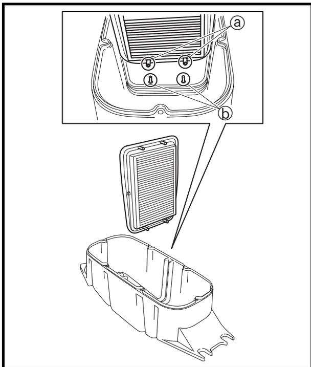
5. Remove the air filter element and check it for dirt and oil. Replace the air filter element if there is any oil buildup.
