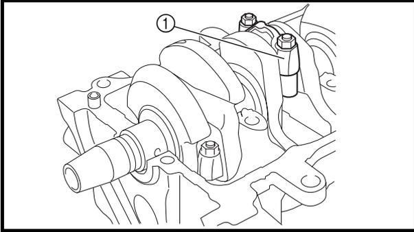
**SERVICE POINTS****Connecting rod and piston removal**
