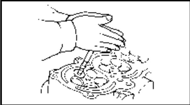
3. Lap the valve slowly on the valve seat with a valve lapper (commercially available) as shown.
