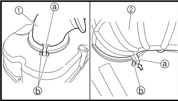
**Air filter case assembly installation**
