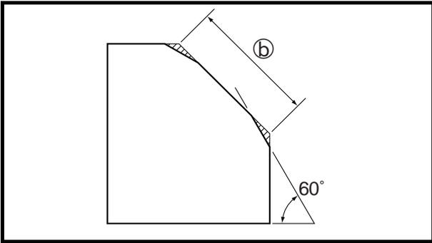
4. Use a 60° cutter to adjust the contact width of the bottom edge of the valve seat.
