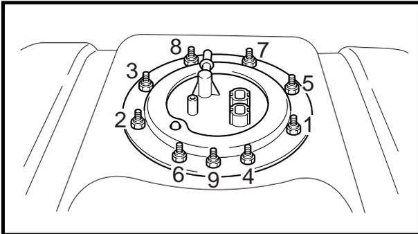
**Fuel pump module removal**
