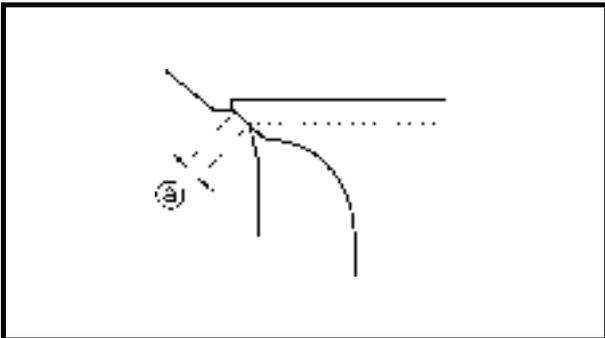
4. Measure the valve seat contact width <sup>Ⓐ</sup> where the blueing dye is adhered to the valve face. Reface the valve seat if the valve is not seated properly or if the valve seat contact width is out of specification. Replace the valve guide if the valve seat contact is uneven.
