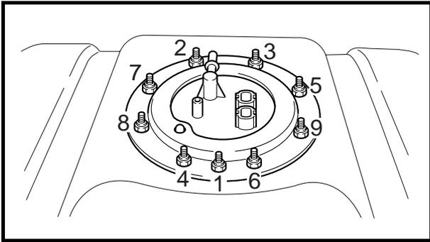
**Fuel pump module installation**
