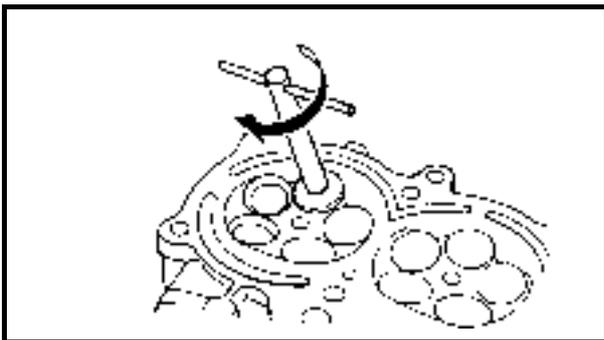
2. Cut the surface of the valve seat with a 45° cutter by turning the cutter clockwise until the valve seat face has become smooth.
