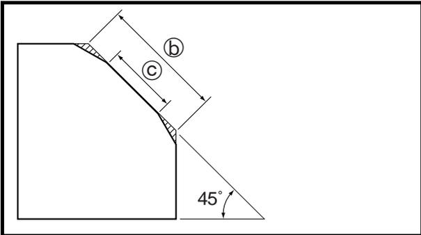
5. Use a 45° cutter to adjust the contact width of the valve seat to specification.
