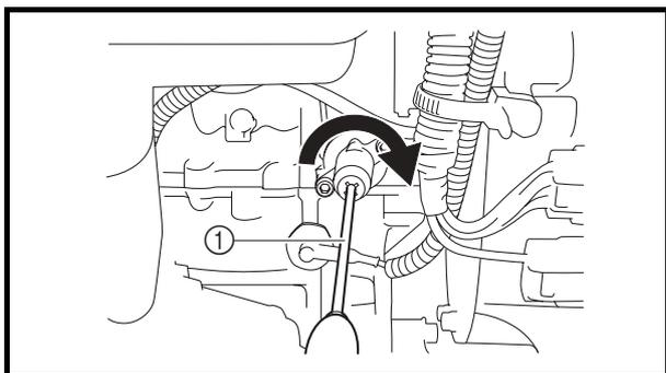
5. Turn the timing chain tensioner rod fully clockwise with a thin screwdriver ①.
