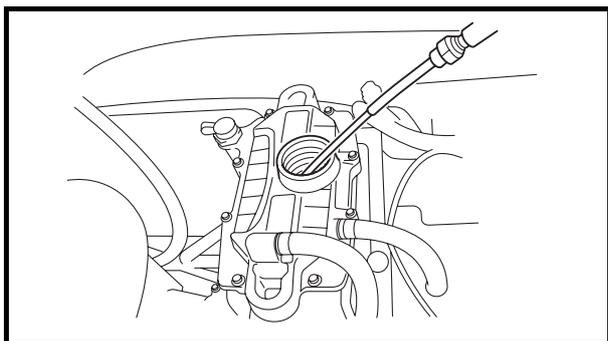
3. Insert the tube of an oil changer into the oil filler hole.
