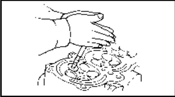
9. Apply a thin, even layer of lapping compound onto the valve seat, and then lap the valve using a valve lapper (commercially available).
