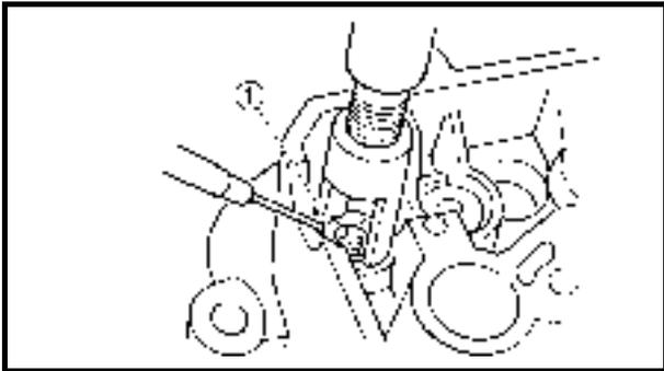
2. Compress the valve spring, and then install the valve cotter ① using a thin screwdriver with a small amount of grease applied to it.
