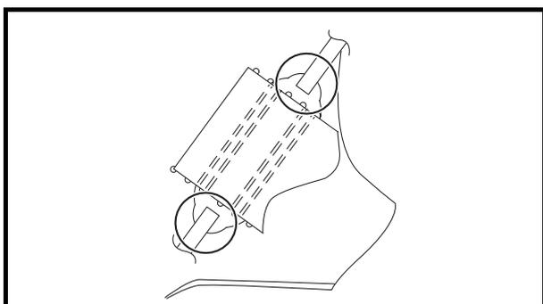
**Ventilation hose assembly installation**
