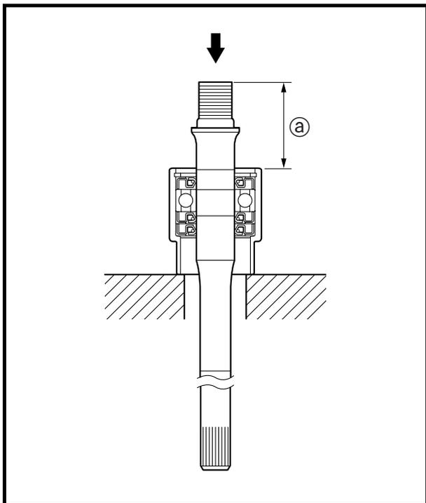
**Intermediate drive shaft installation**
