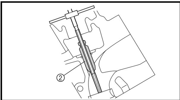
3. Insert the special service tool into the valve guide ②, and then ream the valve guide.
