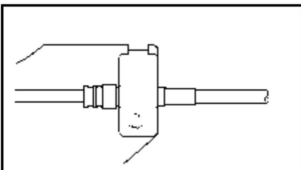
**Steering cable stopper installation**
