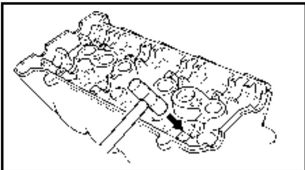
3. Lightly tap the valve spring retainer with a plastic hammer to set the valve cotter securely.
