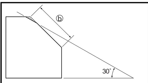
3. Use a 30° cutter to adjust the contact width of the top edge of the valve seat.
