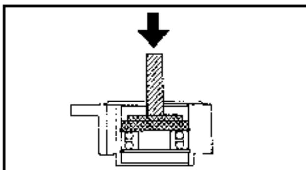
**Bearing removal and installation**
