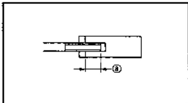
**Jet pump side cable joint installation**
