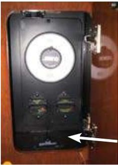
Your boat is equipped with a high bilge water alarm. If the sensors detects high bilge water, an alarm sounds. The most likely causes of high bilge water are: a hull breach, faulty bilge pump or faulty seacock/hose. Immediately identify and correct the cause of the high water, and remove the water. Silence the alarm by turning its circuit switch OFF. The switch is located on the bottom of the Main Cabin DC Access.
