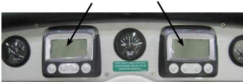
***The engine manufacturer has established a minimum oil pressure rating for your engines, as listed in the engine OEM information. To avoid damaging the engines, shut them off if the oil pressure is below the minimum rating.***
