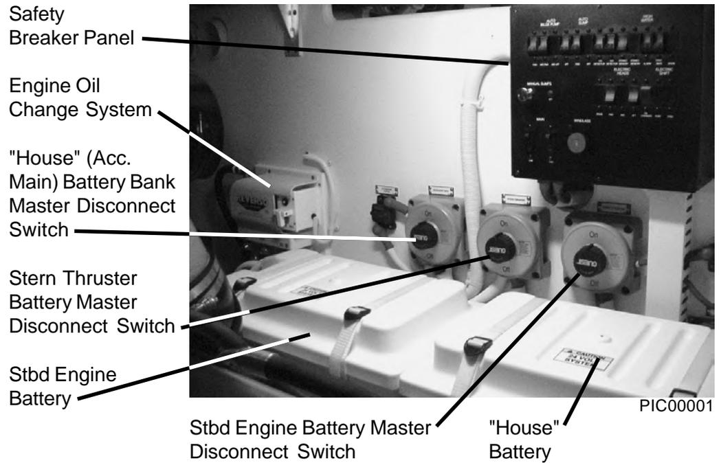
AFT OF STARBOARD ENGINE
