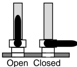
1. Open the overboard discharge seacock located in the engine room just aft of the starboard fuel tank. Refer to **9.7.4 Engine Room** for the exact location of the seacock.
