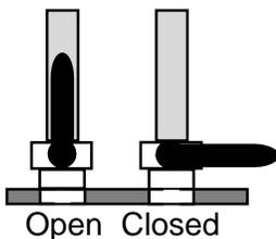
5. Open the cooling system’s seacock.
