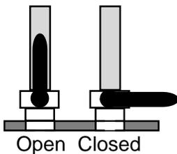
1. Open the cooling system seacocks for both engines.
