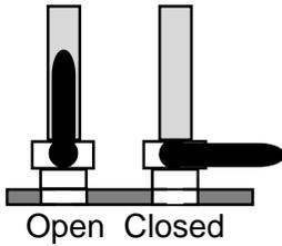
1. Close the seacock that supplies the raw water washdown pump with seawater.
