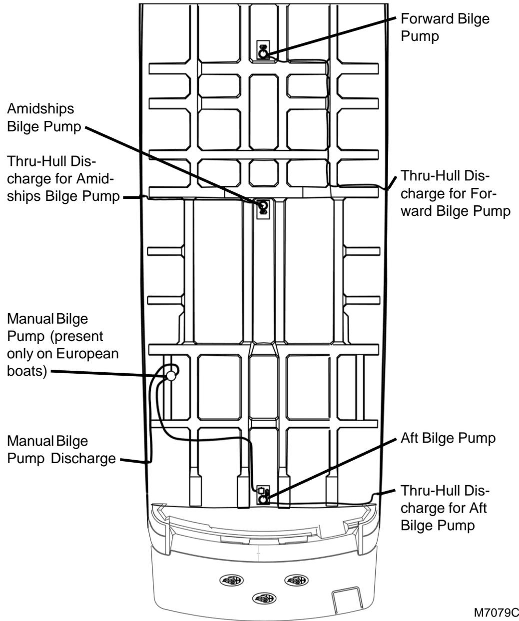
Your boat is equipped with two high bilge water sensors, located above the forward and aft bilge pumps. If one or both of the sensors detects high bilge water, an alarm sounds. The most likely causes of high bilge water are:
