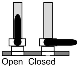
6. Open the washdown seacock to supply seawater to the washdown pump.
