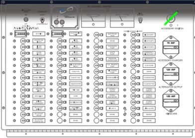
The DC Control Panel manages the power supply to the DC components listed on the panel. The DC panel is located in a cabinet in the aft PORT corner of the salon, and contains the circuit breakers described in this section. The panel also contains additional controls and meters, described in the vendor literature.
