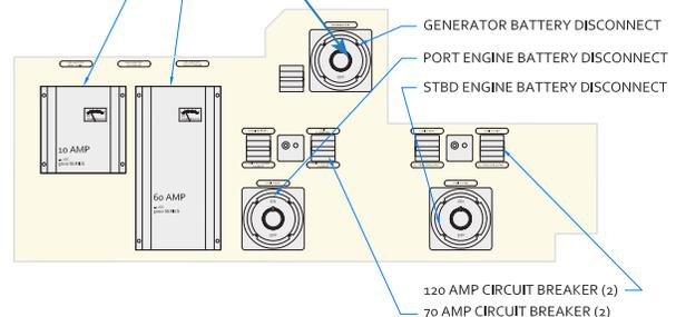
**STEP 11:** To change the AC power source from the generator to shore power, switch the GENERATOR circuit breaker group **OFF**, located on the AC Control Panel. The AC Control Panel is located in the Salon aft STBD Cabinet.
