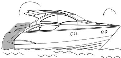
The *station wagon effect* or back drafting can cause CO gas to accumulate inside the cabin, cockpit and bridge areas when operating the boat at a high bow angle or with improper or heavy loading.
