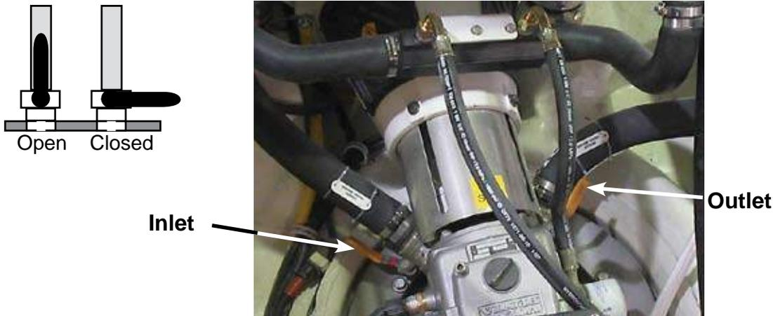
Clean the seawater strainer (located on the left front of the engine) every 14 days or sooner as conditions warrant.
