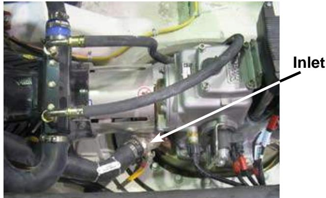
Clean the seawater strainer (located on the left rear of the engine) every 14 days or sooner as conditions warrant.
