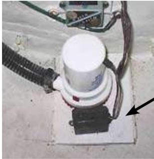
**Note:** *Periodically test each bilge pump by placing two moist fingers on the two round raised areas located on the inside of the switch. The switch is located next to the pump. The pump should turn on after a few seconds of finger contact.*
