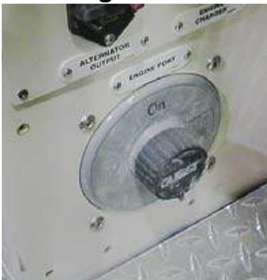
Each propulsion engine has its own battery. Electricity from each battery to its engine is controlled by a master disconnect switch. These switches are located in the engine room near the base on the aft bulkhead. To provide electricity to the engines, turn the master disconnect switches to the ON position. (Port switch shown)
