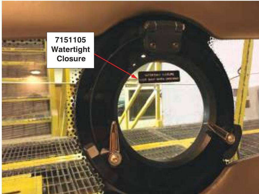
Figure 2-14 – Label Required on all Opening Port Holes
