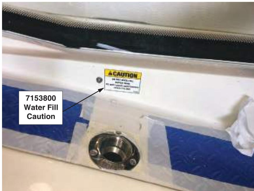
Figure 2-11 – Caution Label at Water Fill Deck Plate
