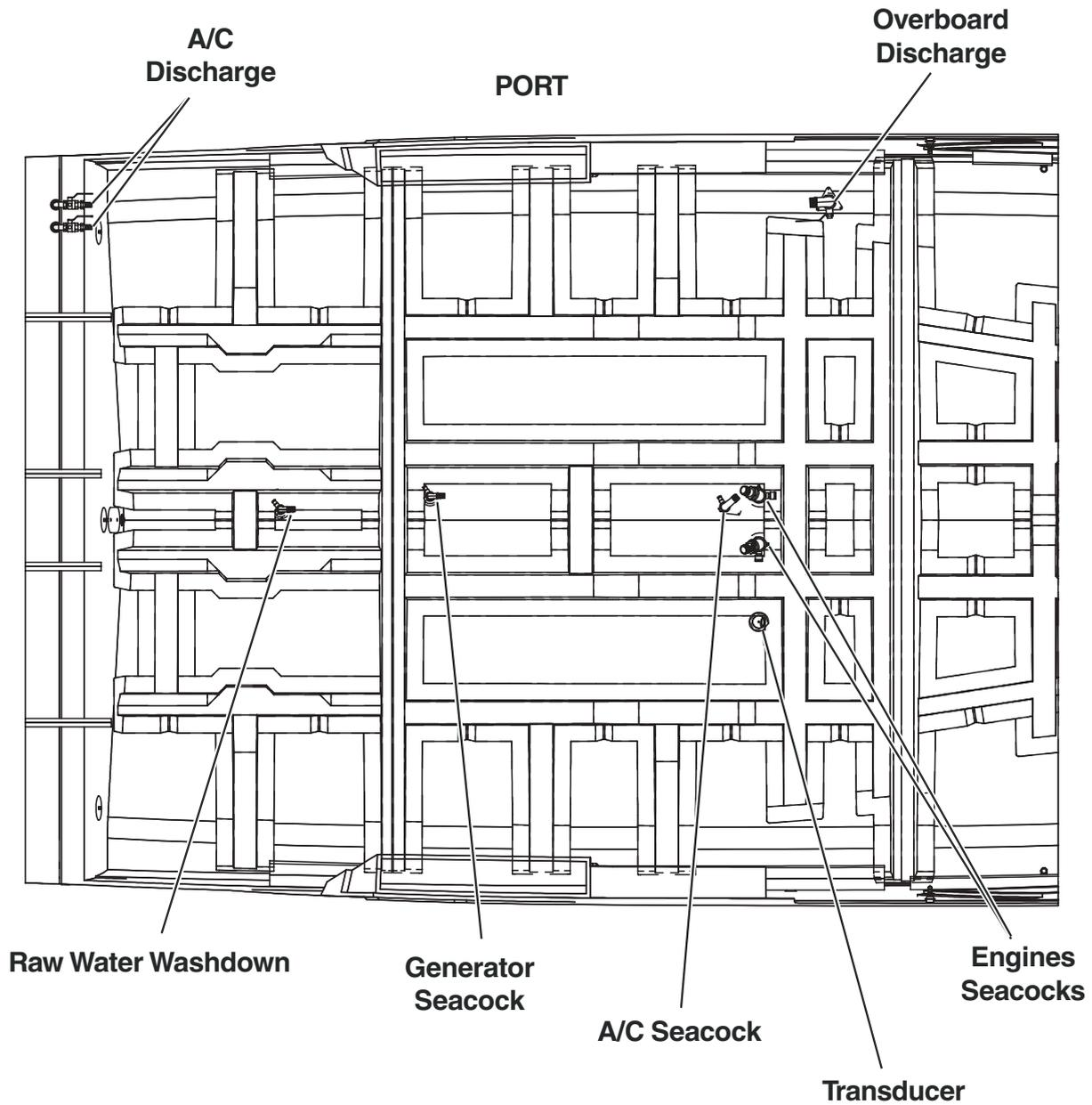
Figure 9-3 – Aft Thru-hull Valves
