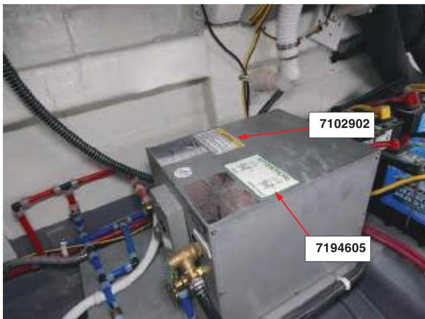
Figure 2-17 – Labels Applied to Top of Water Heater
