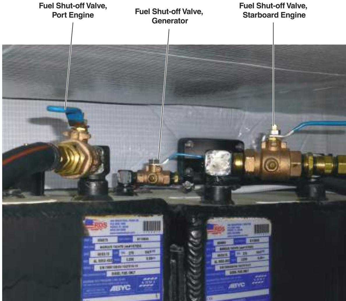
Figure 7-29 – Typical Fuel Shut-Off Valves Installation
