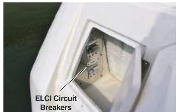
Figure 7-9 – Shore Power Circuit Breakers
