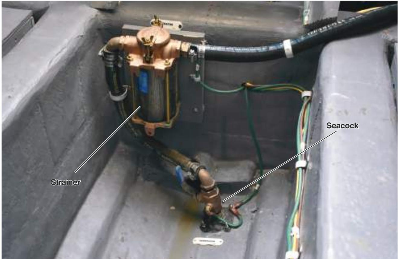
Figure 7-15 – Generator Seawater Strainer and Seacock
