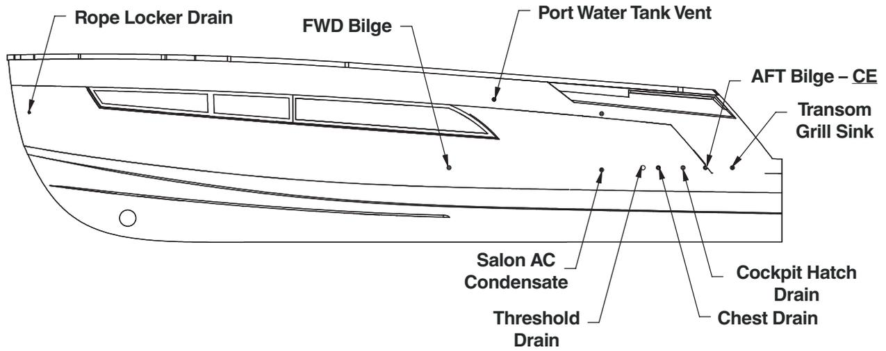
Figure 9-2 – Port Thru-Hull
