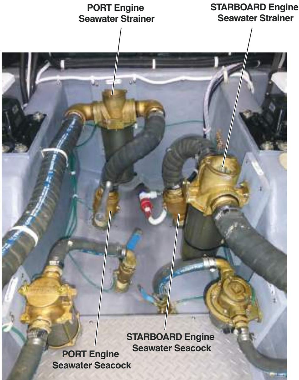
Figure 7-32 – Typical Installation
