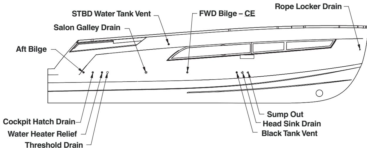
Figure 9-1 – Starboard Thru-Hull
