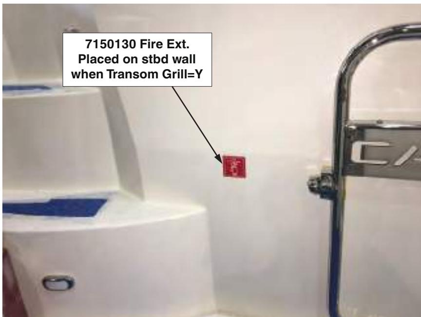
Figure 2-5 – Fire Extinguisher Lable Placed in Cockpit When Transom Grill=Y
