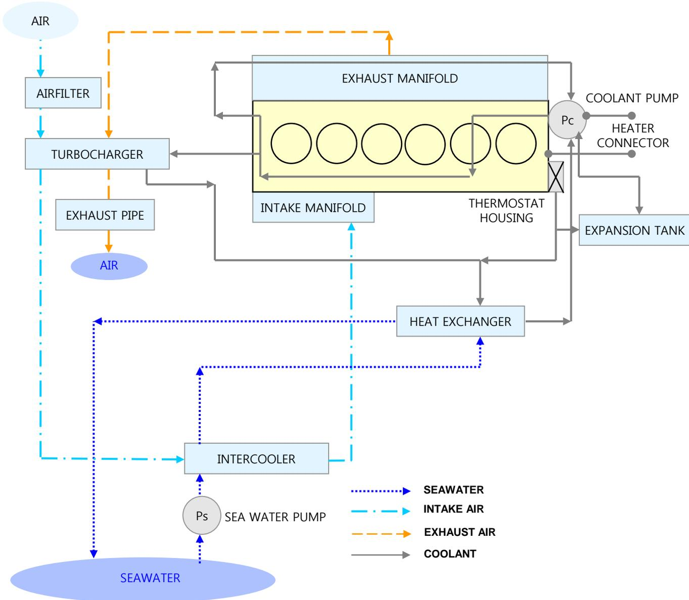
**SEAWATER FLOW – OPEN COOLING CIRCUIT**
