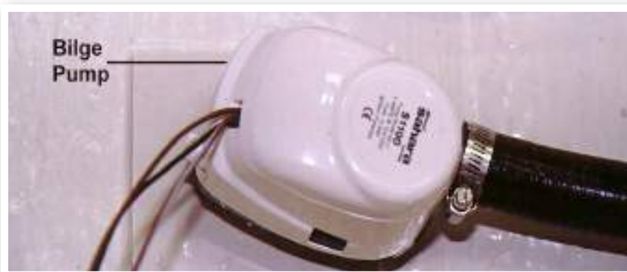
The Bilge Pump is Mounted to ABS Plastic
