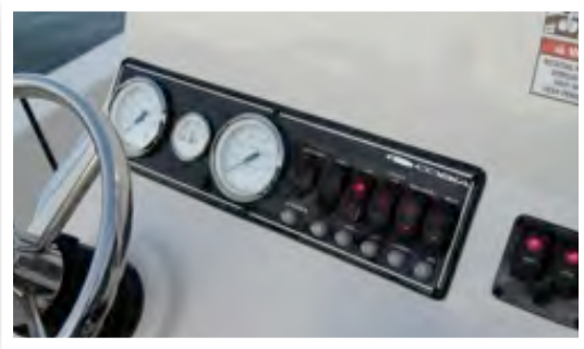
Switch Panel (above)
