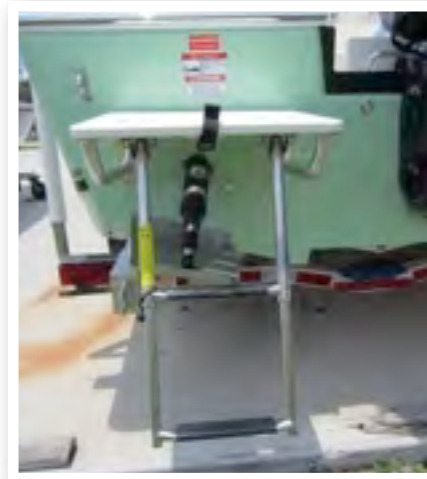
Boarding Ladder ,Extended
