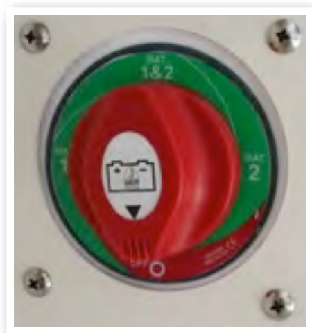
Battery Switch, Shown in the “Off” Position
