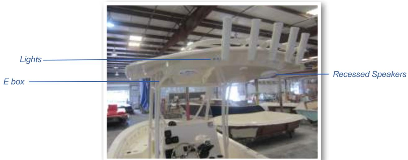
*Fiberglass T-Top with E Box and Speakers*
