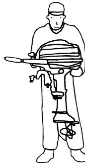
To carry the outboard motor, hold it by the carrying handle, or hold by the carrying handle and the lug beneath the engine cover lock lever, as shown.
