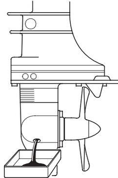
1. Place a suitable container below the oil drain hole to catch the used oil, then remove the oil level screw and oil drain/fill screw.
