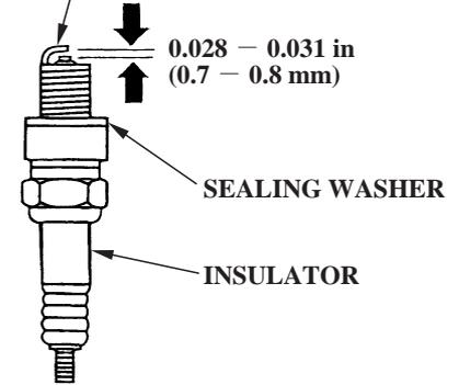
5. Measure the spark plug electrode gap with a wire-type feeler gauge. Correct the gap, if necessary, by carefully bending the side electrode.
