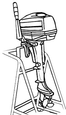
Store the outboard motor either vertically or horizontally with the tiller handle side up.
