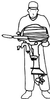
To carry, hold the outboard motor by the carrying handle, or hold by the carrying handle and the lug beneath the engine cover lock latch, as shown.
