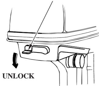
1. Unlock and remove the engine cover.
