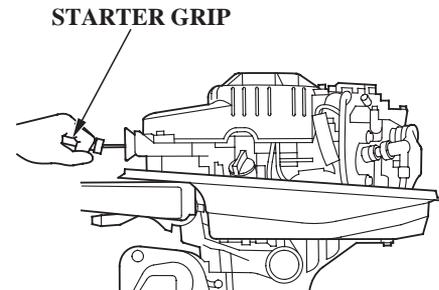
4. Remove the spark plug (p. 49), and remove the emergency stop switch clip from the emergency stop switch. Pull the starter grip, rotate the flywheel a few revolutions to completely expel any water from the cylinder.
