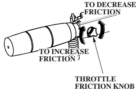
The throttle friction knob adjusts resistance to throttle grip rotation.
