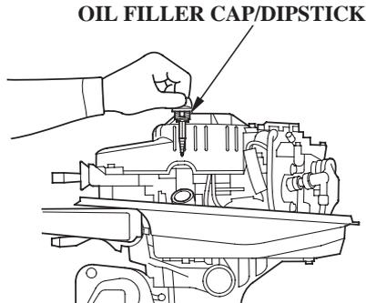
3. Insert the dipstick without screwing it in, then remove it and check the oil level shown on the dipstick.
