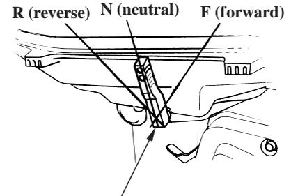
The gearshift lever is used to select F (forward), N (neutral), or R (reverse) gears.
