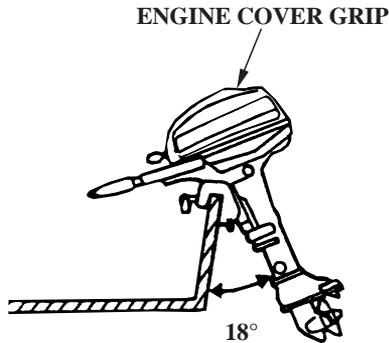
To tilt the outboard motor, raise the outboard motor to the 30° position by pulling on the engine cover grip.
