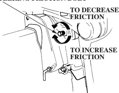
Use the steering friction bolt to help hold a steady course while cruising.
