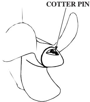
1. Install the shear pin and the propeller, then install the propeller cap finger tight.
