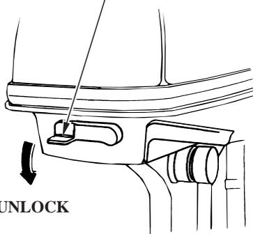
1. Unlock and remove the engine cover for access to the fuel pump filter.
