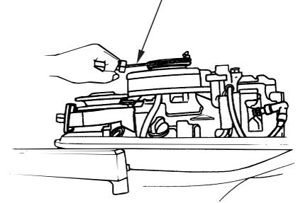
5. Pull the emergency starter rope slowly until resistance is felt, then pull briskly.
