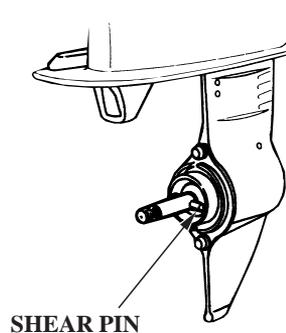
1. Remove the cotter pin, the propeller cap, and the propeller.
