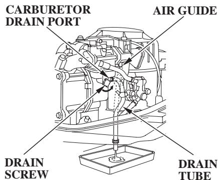
3. With the outboard motor in a vertical position, place an approved gasoline container below the fuel drain outlet, and use a funnel to avoid spilling fuel. Loosen the drain screw to drain fuel from the carburetor.
