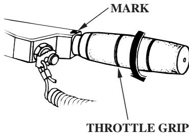
4. Align the START position with the mark for starting the engine.
