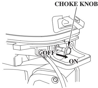
3. To start a cold engine, pull the choke knob to the ON position. To restart a warm engine, leave the choke knob in the OFF position.
