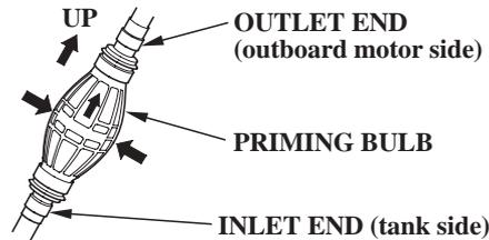
Hold the priming bulb up in the direction of the arrow; then squeeze the priming bulb several times until it feels firm, indicating that fuel has reached the engine.
