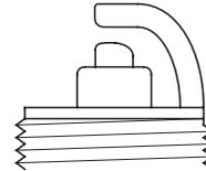
4. Inspect the spark plug. Replace it if the electrode is worn, or if the insulator is cracked or chipped.
