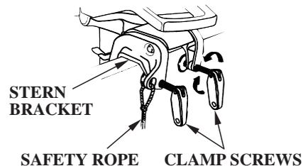
Attach the stern bracket to the boat transom by tightening the clamp screws.
