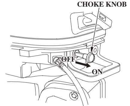
The choke knob opens and closes the choke valve in the carburetor.
