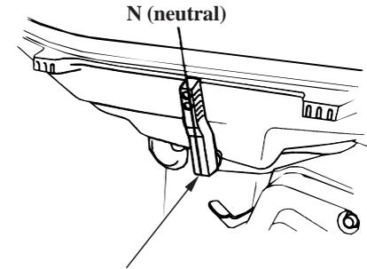
2. Check the position of the gearshift lever. It must be in the N (neutral) position for starting.
