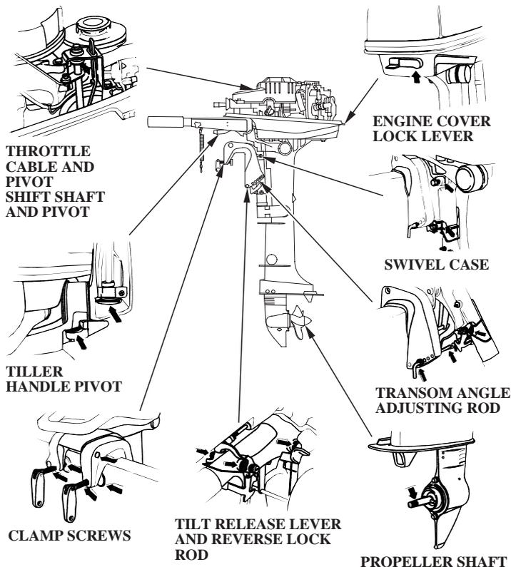
Apply Honda Marine Corrosion Inhibitor (or equivalent) to all areas under the engine cover and any exposed metal surfaces.
