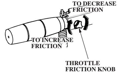
Use the throttle friction knob to help hold a constant throttle setting while cruising.
