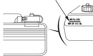
After refueling, install the cap and tighten it until you hear it click. Close the vent by turning the vent knob clockwise all the way, and return the fuel tank to the boat.
