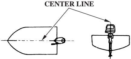
Install the outboard motor on the center of the boat transom.
