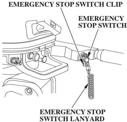
1. Put the emergency stop switch clip in the emergency stop switch, and attach the emergency stop switch lanyard securely to the operator or to the operator's PFD (Personal Flotation Device).
