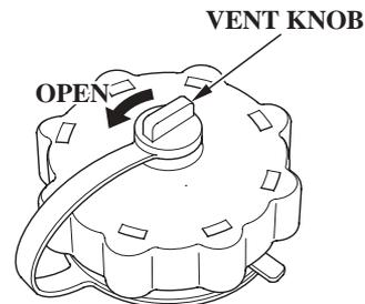
2. Turn the fuel filler cap counterclockwise so that it touches the pressure relief tab.
