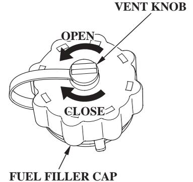
The fuel filler cap is provided with a vent knob to seal the portable fuel tank for carrying it to and from the boat. Open the vent by turning the vent knob counterclockwise all the way before starting the engine.
