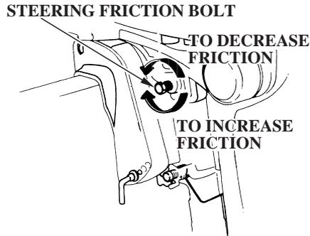
The steering friction bolt adjusts steering resistance.
