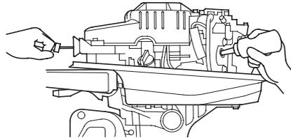
5. Pour a teaspoon of engine oil into the spark plug hole, and then pull the starter grip several times to lubricate the inside of the cylinder.
