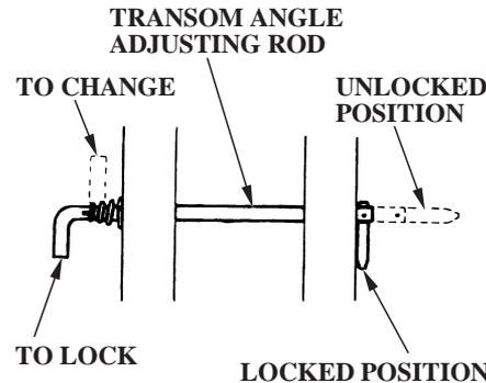
The transom angle adjusting rod is used to adjust the angle of the outboard motor in the normal operating position (p. 35 ).
