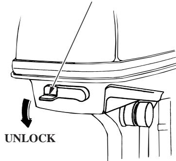
The engine cover lock lever fastens the engine cover to the outboard motor.
