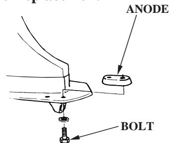
The anode is located on the antiventilation plate. It is made of a sacrificial material that helps to protect the outboard motor from corrosion.
