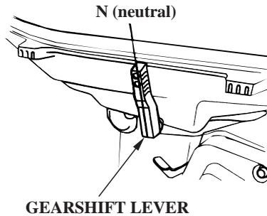
1. Move the throttle grip to the slowest speed and gearshift lever to the N (neutral) position.
