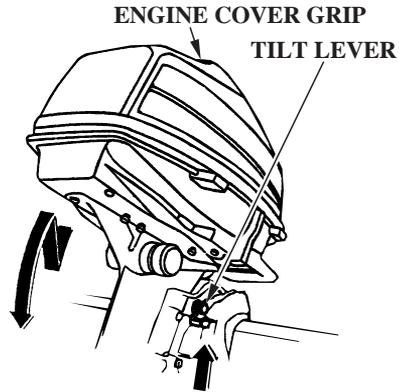
The tilt lever enables the outboard motor to be raised for shallow water operation, beaching, launching, or mooring.
