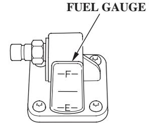
A fuel gauge is built into the fuel tank connector of the portable fuel tank.
