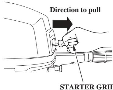
5. Pull the starter grip lightly until you feel resistance, then pull briskly in the direction of the arrow as shown above.
