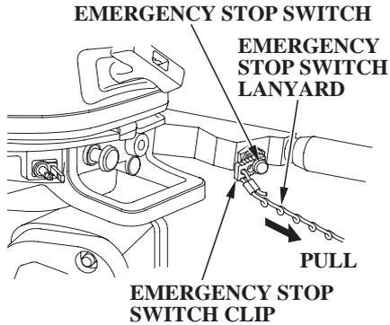
To stop the engine in an emergency, pull the emergency stop switch clip out of the emergency stop switch by pulling the emergency stop switch lanyard.
