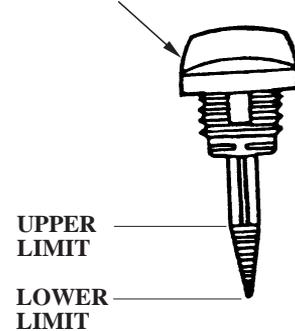
4. If the oil level is low, add oil to reach the upper limit mark shown on the dipstick. Use the oil recommended on p. 45.
