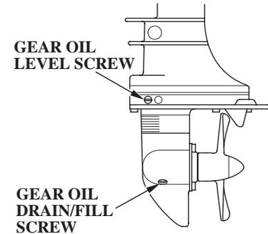
Remove the oil level screw and see whether oil flows from the oil level hole.
