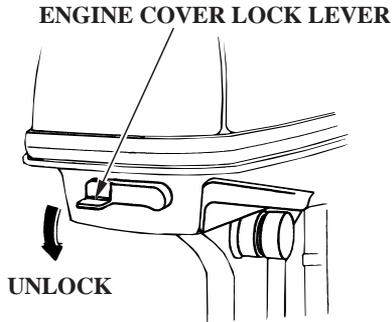
The engine cover lock lever fastens the engine cover to the outboard motor.
